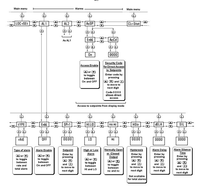
Fig 13 Alarm menu structure
