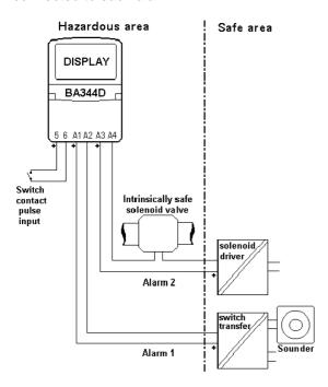
Fig 12 Typical alarm application
