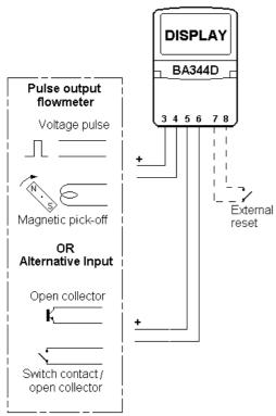
Fig 2 Stand alone operation within hazardous area
