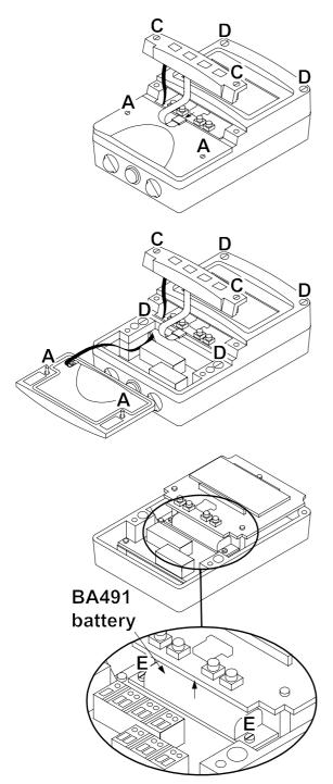
Fig 7 Replacement of internal battery
