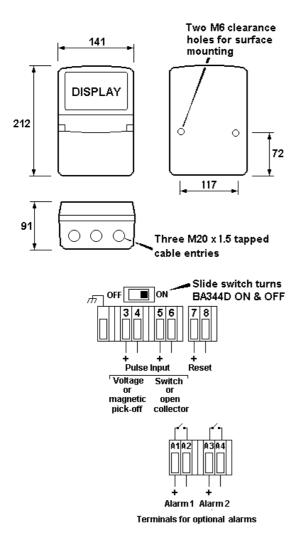
Fig 6 Dimensions and terminal connections
