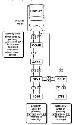
Fig 14 Setpoint adjustment from the display mode
