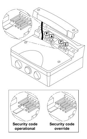
Fig 10 Location of security override link & function of push-buttons
