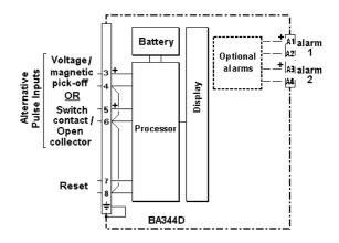
Fig 1 Simplified block diagram of BA344D
