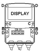
Install cable glands, conduit fittings or blanking plugs and terminate field wiring. If the instrument is about to be commissioned put the ON / OFF switch in the ON position. Finally replace the terminal cover and
