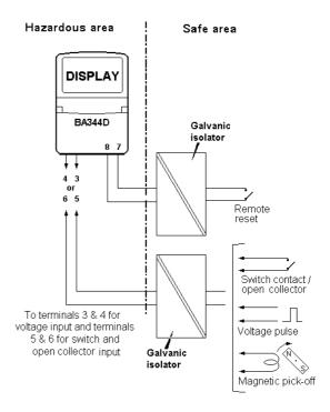
Fig 4 BA344D used with galvanic isolators
