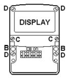
Secure the instrument to a flat surface with M6 screws through the two 'B' holes.
